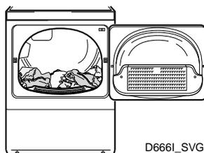
4. Close loading door. Dryer will not operate with the door open.
